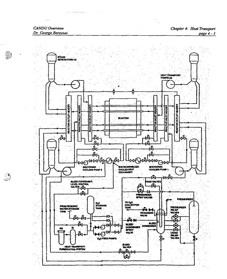
Figure 4.1. Heat Transport Systems Simplified Composite Flow Diagram.
